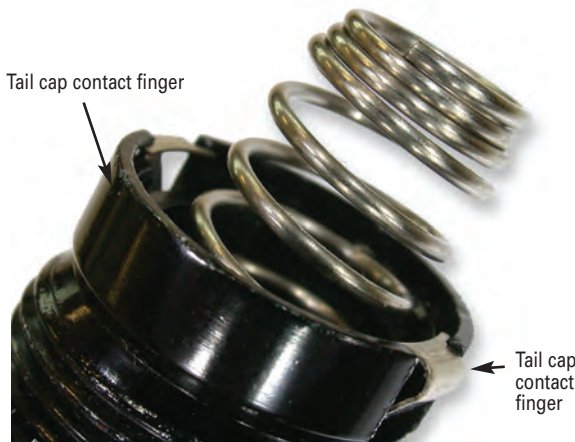
Figure 3 – Tail cap contact fingers – normal condition
