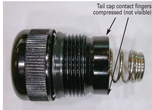
Figure 4 – Tail Cap Contact with compressed fingers
