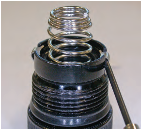
Figure 5 – Using an eyeglass repair tool to force the tail cap contact fingers outward.
