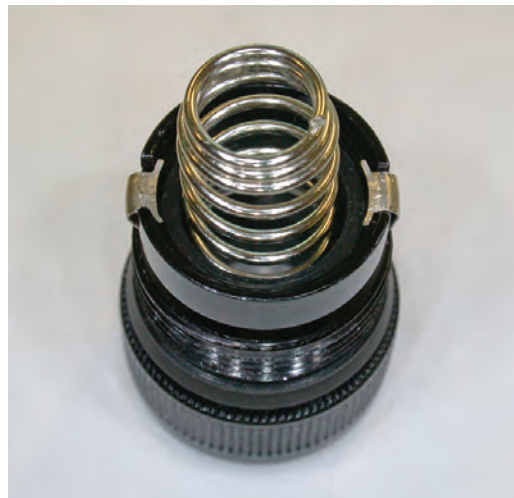
Figure 6 – Tail cap with tail cap contact fingers restored to correct position.
